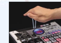
The beam in the photo has been colored to show the path of the D Beam; the actual beam is invisible.
